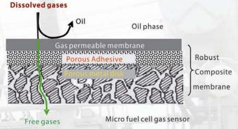
TransPRO® KG1100 is designed for continuous, long-term and on-line monitoring of fault gases dissolved in oil. It is particularly suitable for OEM purpose, or for the user seeking cost-effective early warning device for oil-filled electrical equipment such as transformer or shunt reactor.
