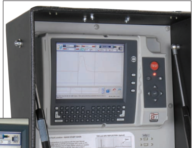
New style MTDR is mounted in the lid for easier viewing with a large, bright screen.
