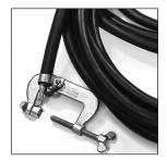
Heavy-Duty C-Clamps — Current passes through the C-clamp and screw thread; the potential passes through a four-point anvil insulated from the clamp metal. This set of leads is available in two widths and a variety of lengths. Cat. No. 242004-7, 242004-18, 242004-30, 242104-2-16, 242104-2-26
