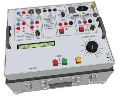
The 100ADM mk4 provides commissioning and maintenance engineers with a flexible system for testing protective systems. It has an easy to understand panel layout and a simple user interface. The status of every function can be seen at a glance, and there are no complex menus to navigate.
